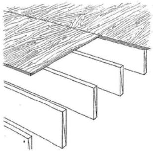
**Description:** Table below lists the S.F. costs for wood joists and a minimum thickness plywood subfloor.
